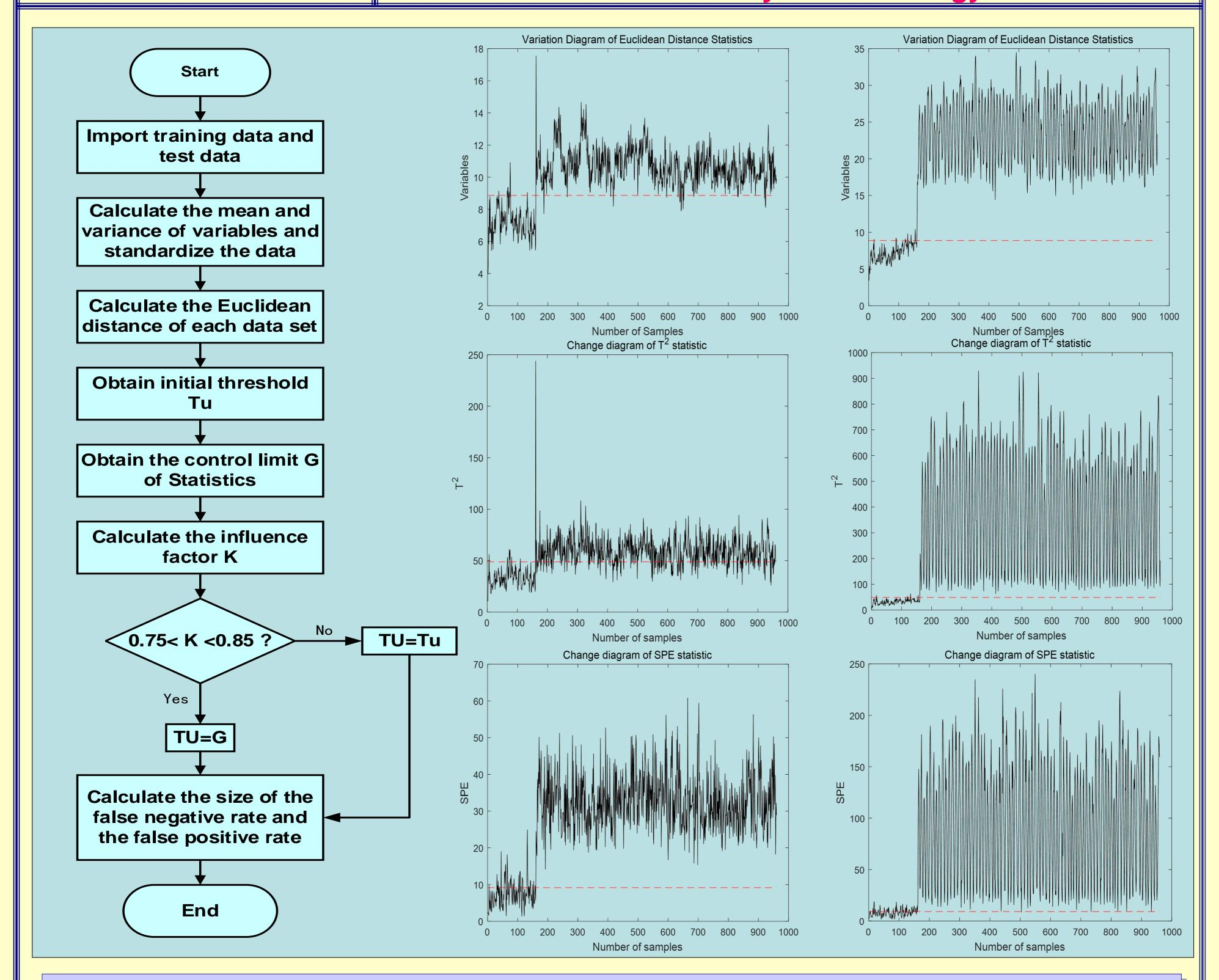
Flow and simulation diagram of fault detection method based on improved Euclidean distance control
