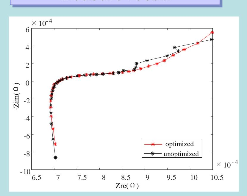
be seen from the can that the optimized figure impedance measured spectrum curve is smoother and the measurement results are more accurate.
