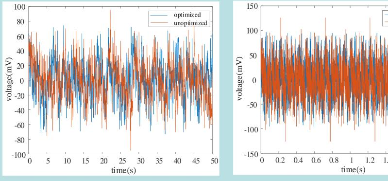
The peak amplitude of the current excitation over frequency bands of 0.1Hz-10Hz and 10Hz-1000Hz is reduced by 22.7% and 23.9% respectively
