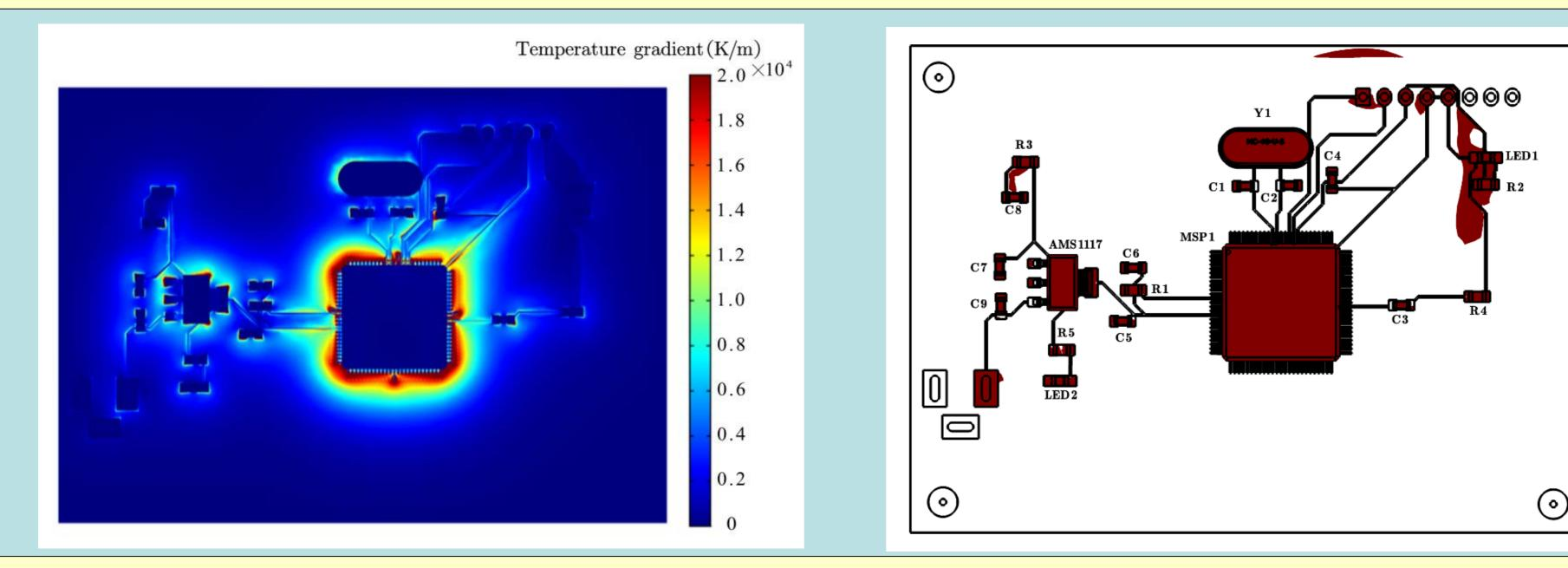
The temperature gradient and feature recognition using the temperature gradient threshold operator on the PCB.
