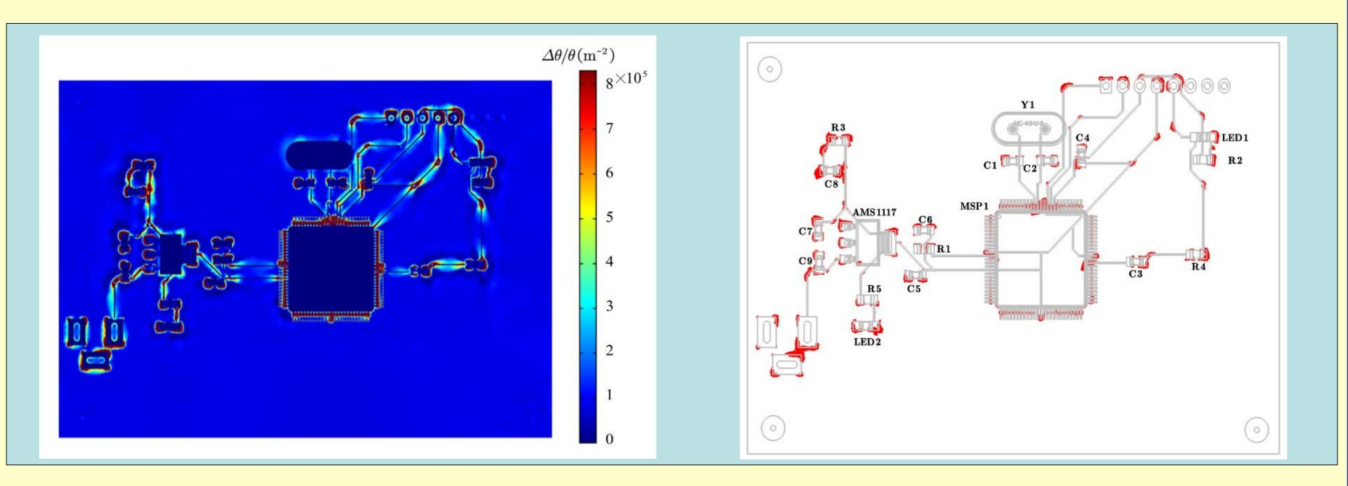
The improved Laplace parameter and feature recognition using the improved temperature Laplace threshold operator on the PCB.
